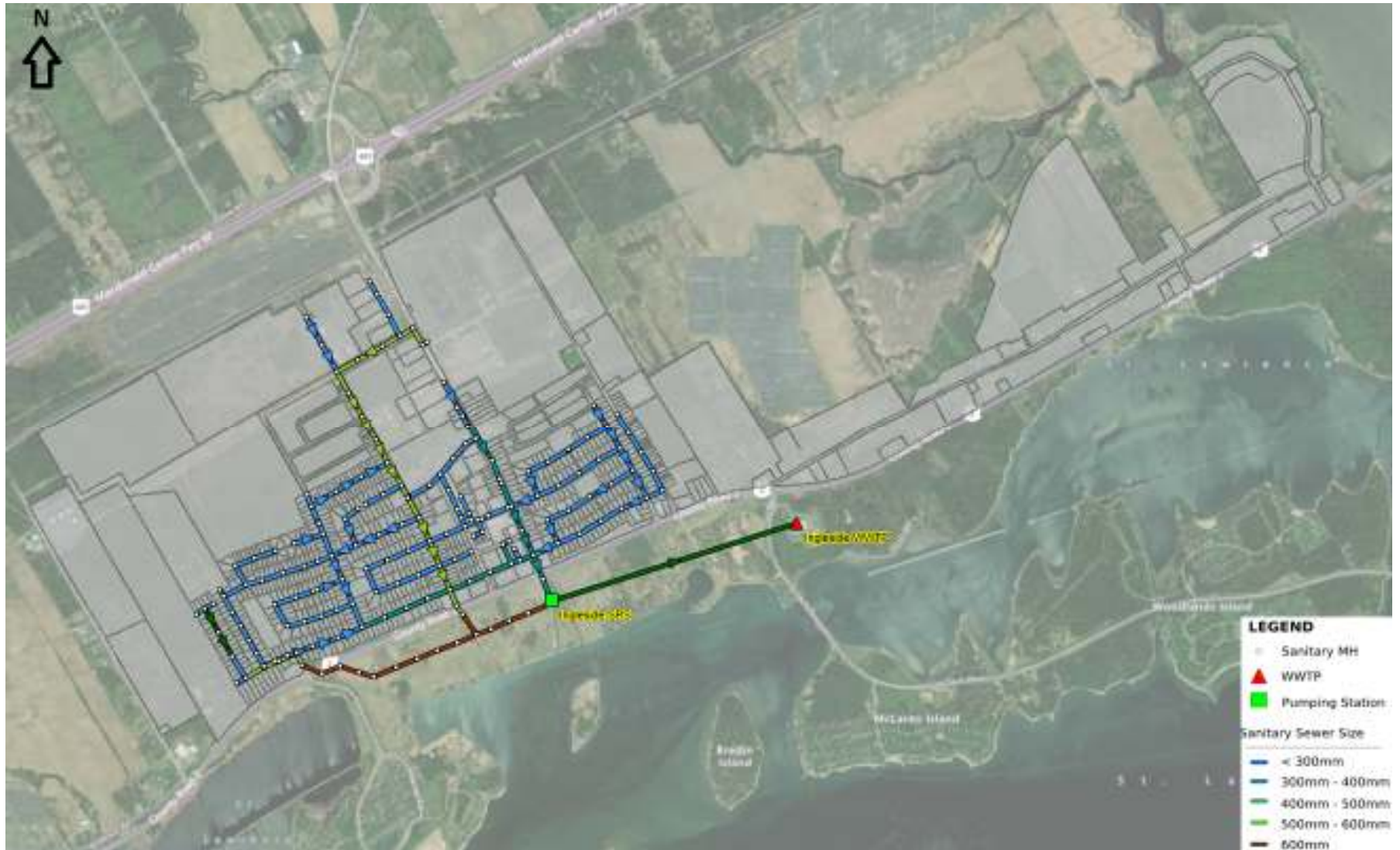
Figure 3-3 Existing sanitary sewer within the Village of Ingleside
