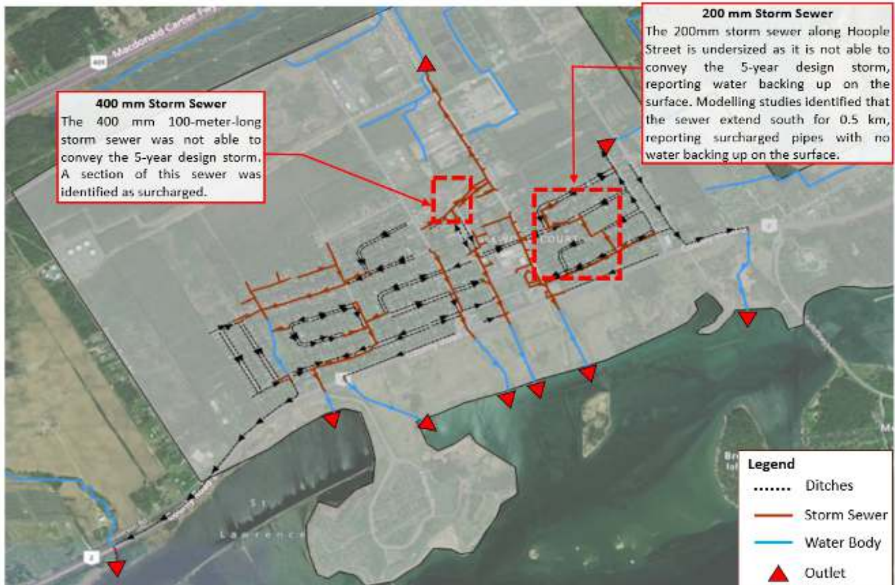
Figure 3-7 Storm Sewer System Limitations
