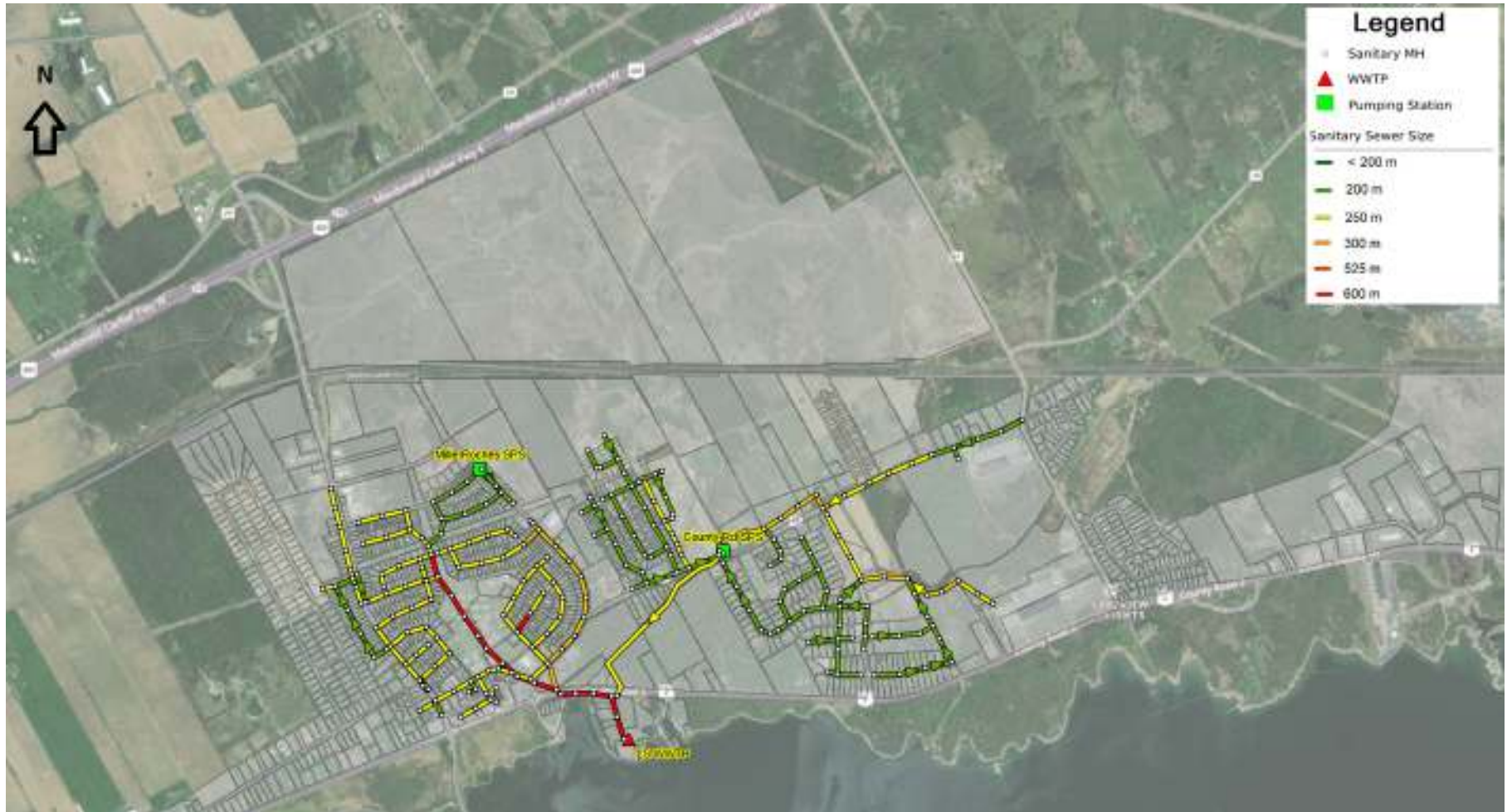
Figure 3-4 Existing sanitary sewer within the Village of Long Sault
