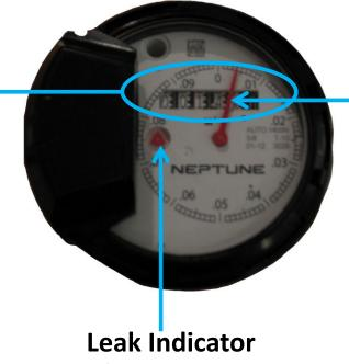
Movement of this triangle when all water fixtures in home are closed suggests a leak
