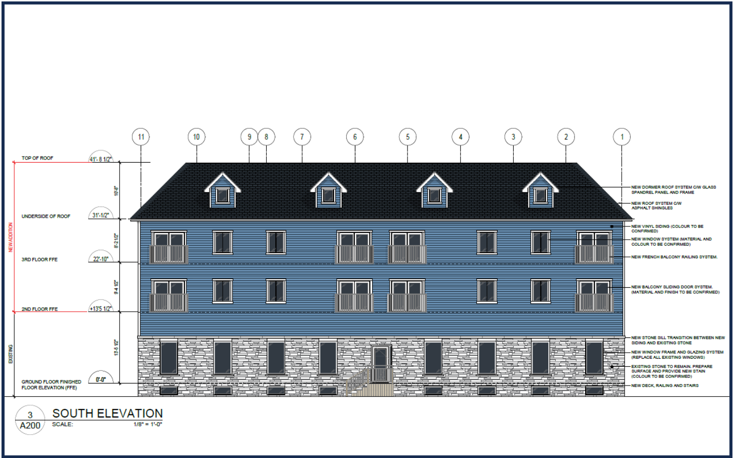
Image 1: Proposed South Elevation of Building
